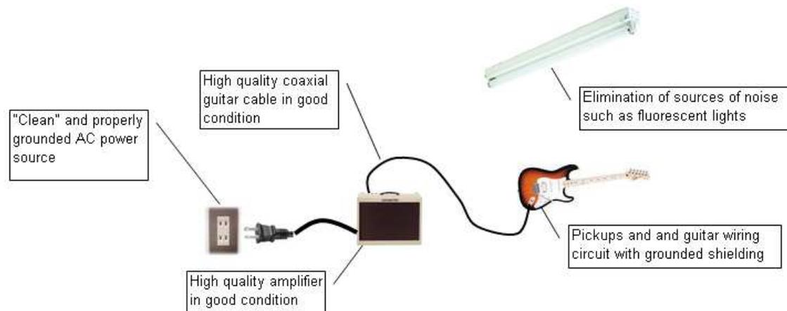
To get the lowest noise possible one must think of the whole system: the electromagnetic environment (noise sources), guitar, guitar cable, amplifier and the AC power supply.
