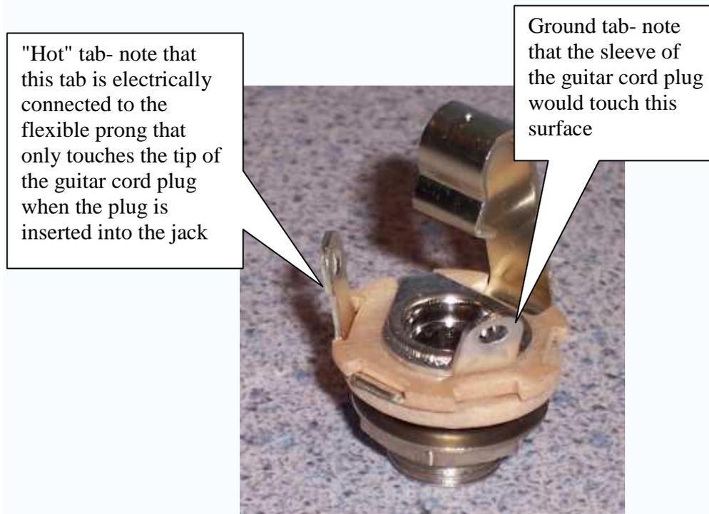
Output jack used commonly used in an electric guitar
